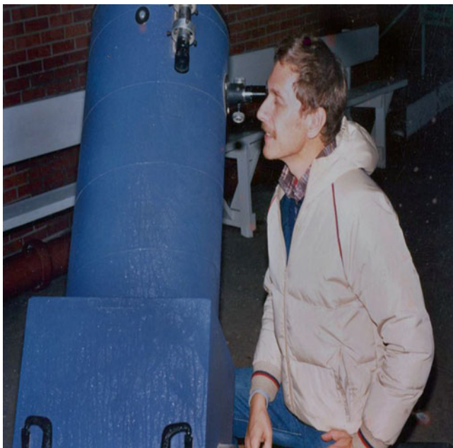
Fig. 1.2 Greg Boles of Topeka, Kansas, is using a 1980s Coulter Optical “Blue” tube “rocker box” style 13.1-in. f/4.5 Dobsonian to observe the heavens with (Image credit: Rick Schmidt)
