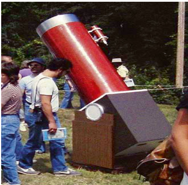
Fig. 1.1 A 1980s Dobsonian style Newtonian “rocker box” housed in an Altazimuth mount (Image credit: Halfblue-Wikipedia)
