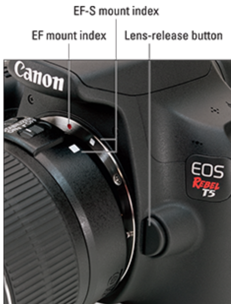
Figure 1-1: Align the mounting index on the lens with the one on the camera body.
