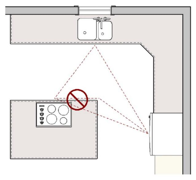
Each leg is measured from the center-front of the appliance/sink.
