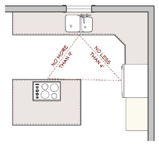
When the kitchen plan includes more than three primary appliance/work centers, each additional travel distance to another appliance/work center should measure no less than 4' (1.2 m) nor more than 9' (2.7 m).
