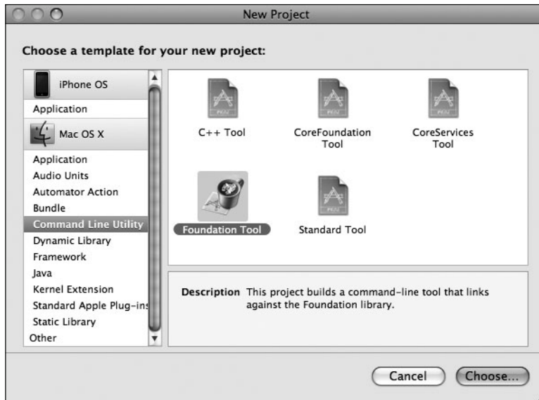
Figure 2-1. Making a new foundation tool
