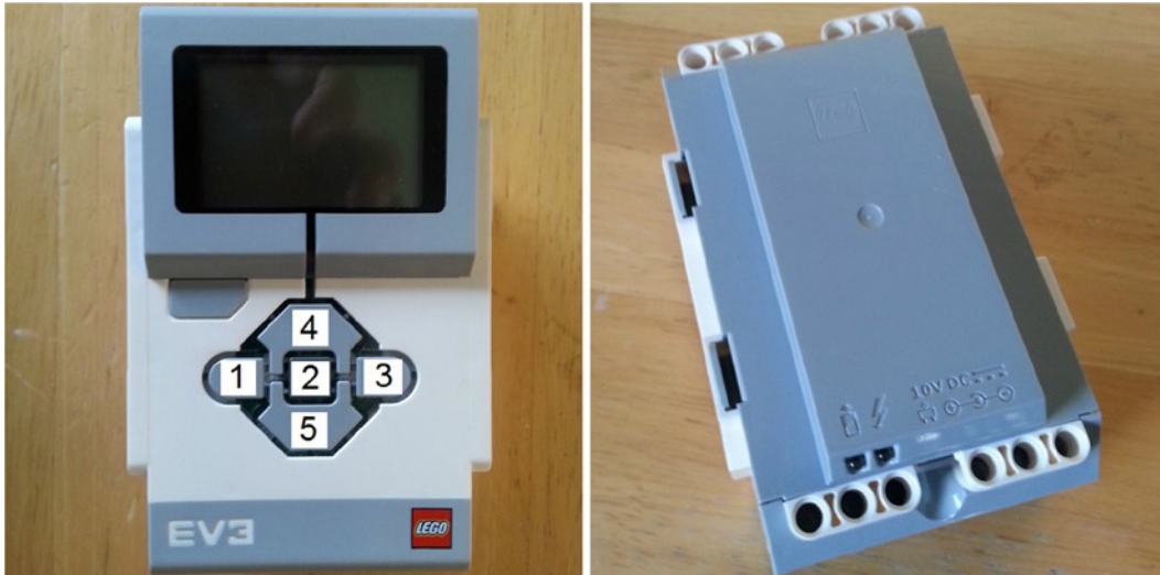
Figure 1-1. Front and back views of the EV3 Brick. The back is the 10V battery
