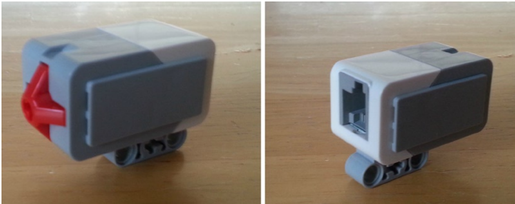
Figure 1-8. The front and back view of a Touch Sensor
