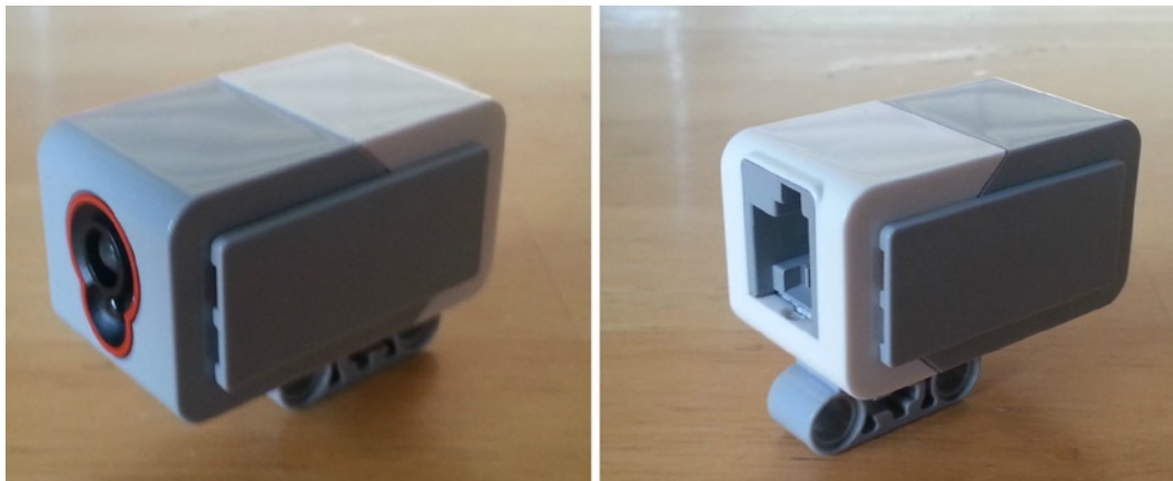
Figure 1-7. Front and back views of the Color Sensor
