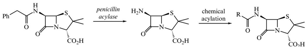
**Figure 1.4** Industrial production of a semi-synthetic penicillin using penicillin acylase.
