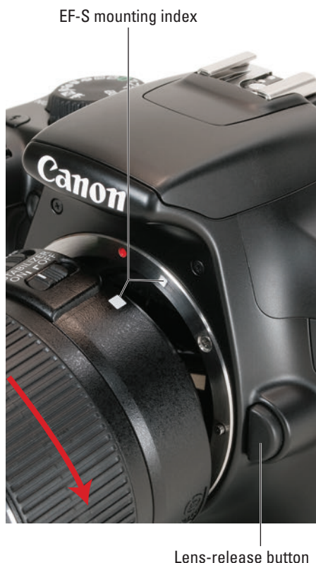
Figure 1-2: Place the lens in the lens mount with the mounting indexes aligned.
