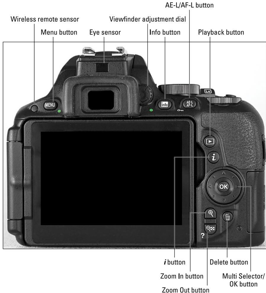
**Figure 1-7:** For quick access to primary picture settings, press the *i* button.
