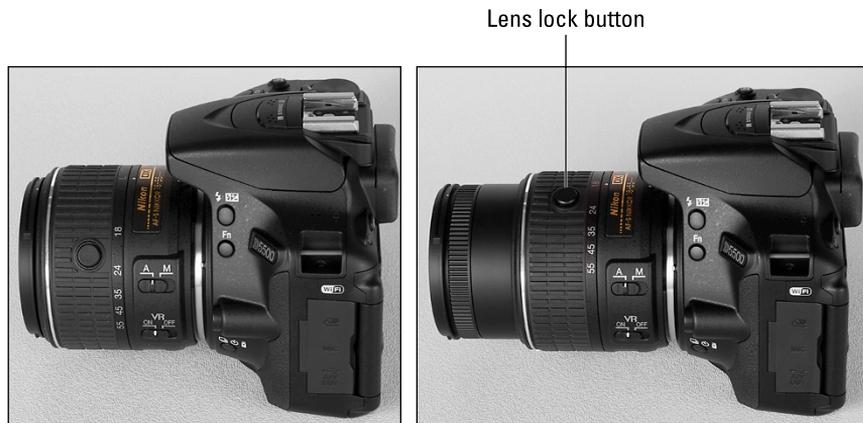
**Figure 1-5:** If using a retractable lens, press the lens lock button while rotating the lens barrel to extend and retract the lens.
