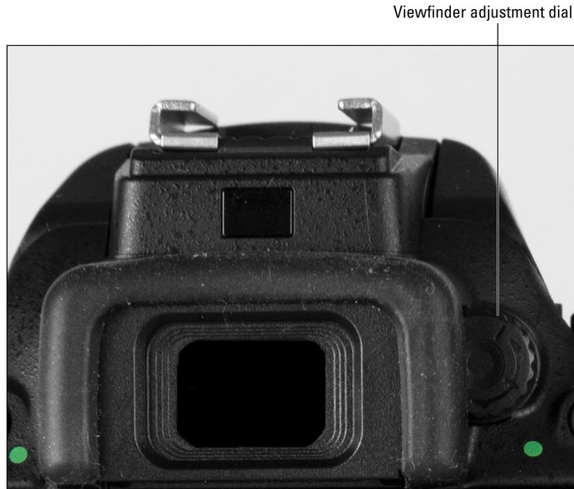
**Figure 1-4:** Rotate this dial to set the viewfinder focus for your eyesight.
