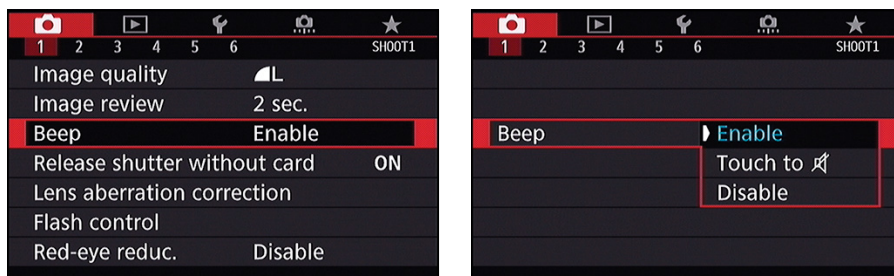
FIGURE 1-11: Set the Beep option to Touch to Silence to prevent the camera from making a sound when you tap a touch-controlled item.
