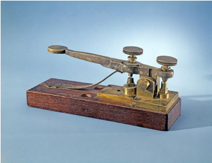
Figure 1-1. Morse-Vail Telegraph Key
